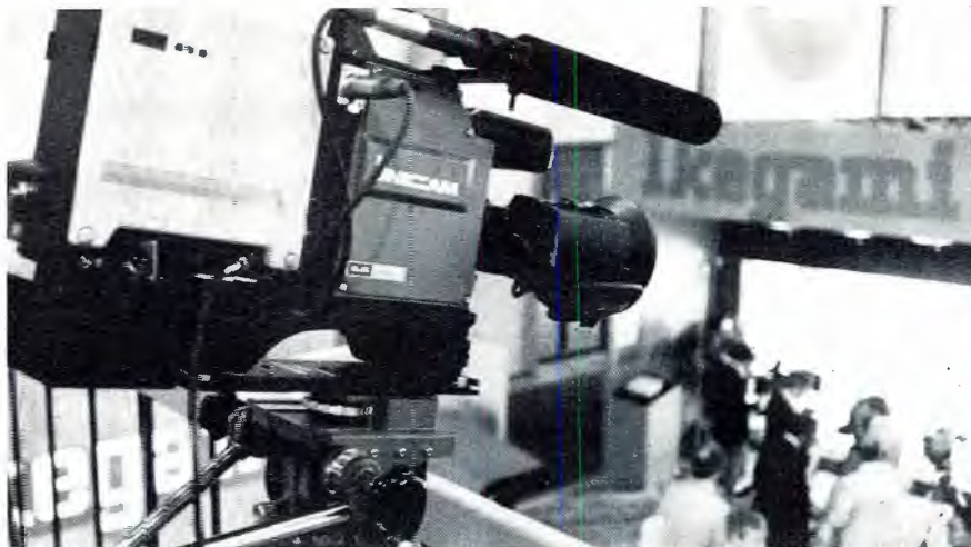
The Ikegami HL-95 camera attaches to a 1/4-inch Hitachi or other format recorders.
